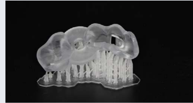
Fig. 7: 3D-printed guide with supports with Primeprint Guide material
