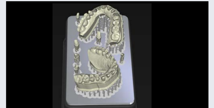
Fig 10: Models and dies on build plate inLab CAM 22
